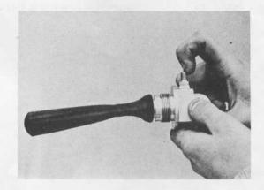
When installing new bladder, depress air valve to allow bladder to assume its natural shape before inserting in shaft.
